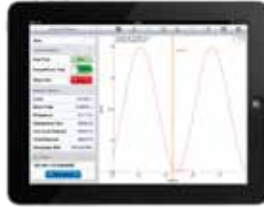
The Spider-81C connects directly to an iPad with a built-in Wi-Fi router.
