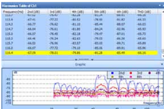
Compute THD of the control and input signals
