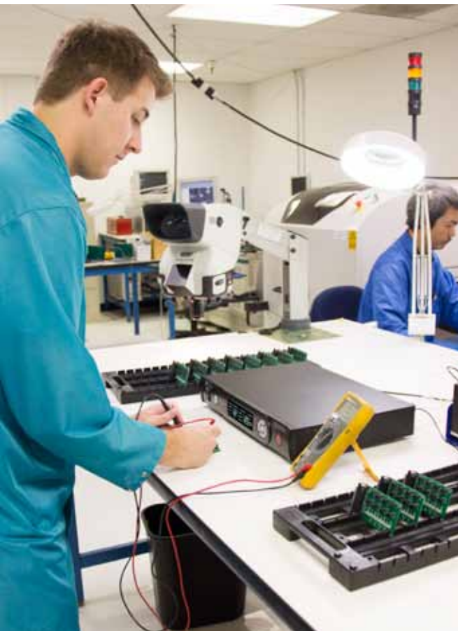
The Spider-81 being used in a “pass/fail” test
