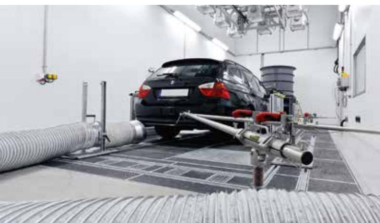
In addition, it permits sunlight simulation at up to 1000 W/m<sup>2</sup>. On the test bench, an airstream blower creates wind with a velocity of up to 120 km/h, proportional to the simulated driving speed.
